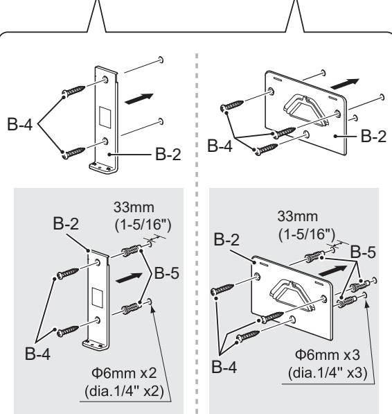
When mounting on a plaster board or tiled wall. /
