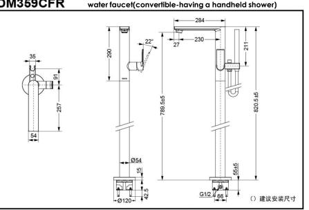
Copper alloy vertical single-handle double-control bath tub
