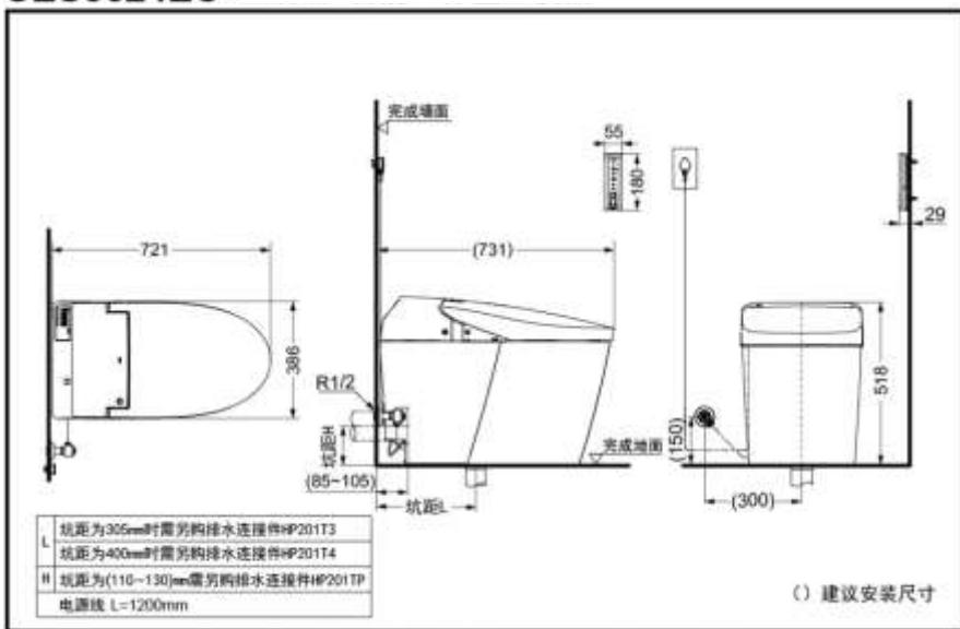
**SPECIFIECS****Size :** 518×386×721mm**Nominal Water :** 3.5L**Dual Flush Volume :** 3.0/4.5L**Water Efficiency :** Grade2**Water Inlet Requirement :**
