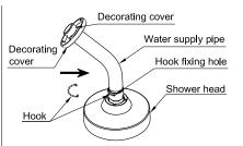
②Hang one end of the hook preventing drop in the fixing hole of the shower head and the other end in the fixing hole on the other end for fixing.
