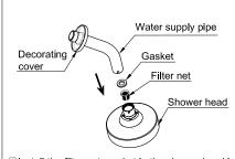
①Install the filter net, gasket in the shower head in proper order and use a wrench to tighten with the water supply pipe.
