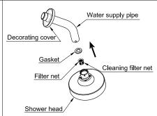
②Open by screwing the shower head and water supply pipe screw threads. Take out the gasket, filter net in proper order. If too much dirt is left on the filter net, clean the filter net.
