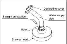
①As shown in the above figure, use a straight screwdriver to align with the gap between the hook and shower head. Just prize lightly for removal. Attention: Please support the hook with hand in removing to avoid the hook falling off and losing and pay attention to safety to avoid the screwdriver injuring hand.
